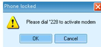
3. After pressing **OK**, you access the Call window. Then dial **\*228** for activation (provisioning on MIN & MDN).
